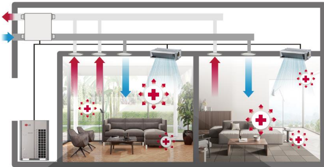
Principle of creating positive pressure
